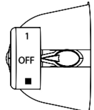
The figures do not mean specific set temperature, but the temperature level.
