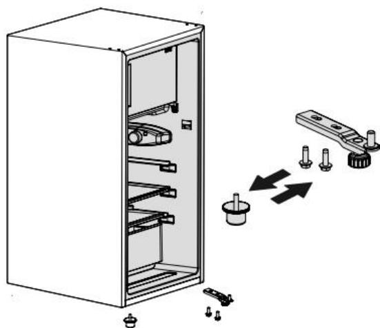
4. Dismantle the stopper under the door, then assemble the stopper on the other side
