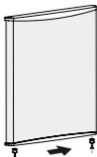
5. Install the door on the lower hinge assembly, and then install the upper hinge, hinge cover, pins and hole cap in sequence.
