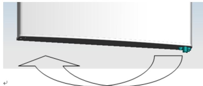
18)Move the lower hinge to the other side and screw it in place.
