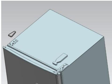
14) Using a cross screwdriver, remove the screws from the upper hinge.
