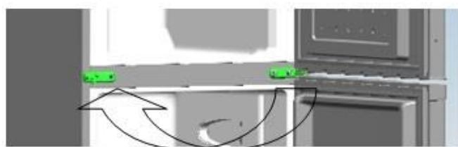
20)Adjust the lower door to the correct position, screw the middle hinge in place.
