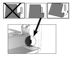
Attach the frame by tightening it with the door. Do not press on the frame alone.
