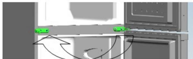
20)Adjust the lower door to the correct position, screw the middle hinge in place.
