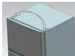
22) Adjust the upper door to the correct position, screw the upper hinge and the cover in place.
