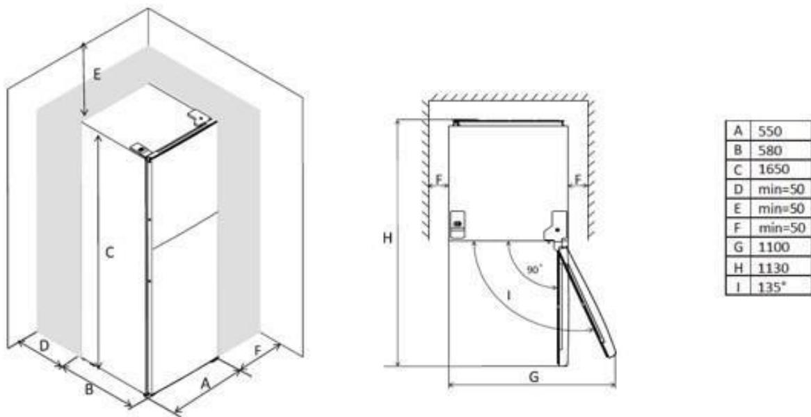
**i** Note that this appliance is not designed for built-in installation.
