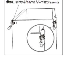
7. Unscrew and remove the bottom hinge pin, turn the bracket over and replace it.
