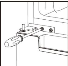
10. Place the upper door back on. Ensure the door is aligned horizontally and vertically so that the seal are closed on all sides before finally tightening the top hinge. Then inert the top hinge and screw it to the top of unit and then fix hinge cover (in accessory bag) by screw.
