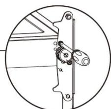
5. Adjusting the hinge core position of the lower hinge and upper hinge to opposite position
