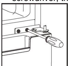
4. Laying down the refrigerator, take out the adjusting feet as below, then take off the lower hinge by cross screwdriver.
