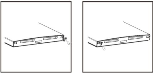
9. Install the lower door, adjust and fix the middle hinge onto the cabinet.
