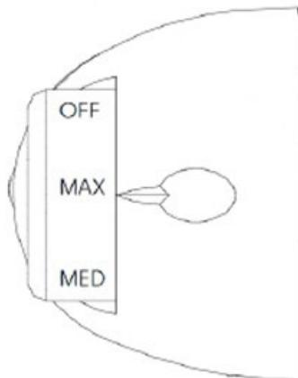
The thermostat control knob is located on the right wall inside the refrigerator.
