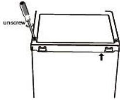
2. Carefully lift the top cover 5 cm away from the freezer, and then pull out the terminal. Then remove the top cover away:
