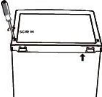
11. With the door closed, check that the door is aligned horizontally and vertically and that the seals are closed on all sides before finally tightening the bottom hinge. Re-adjust the levelling feet as needed
